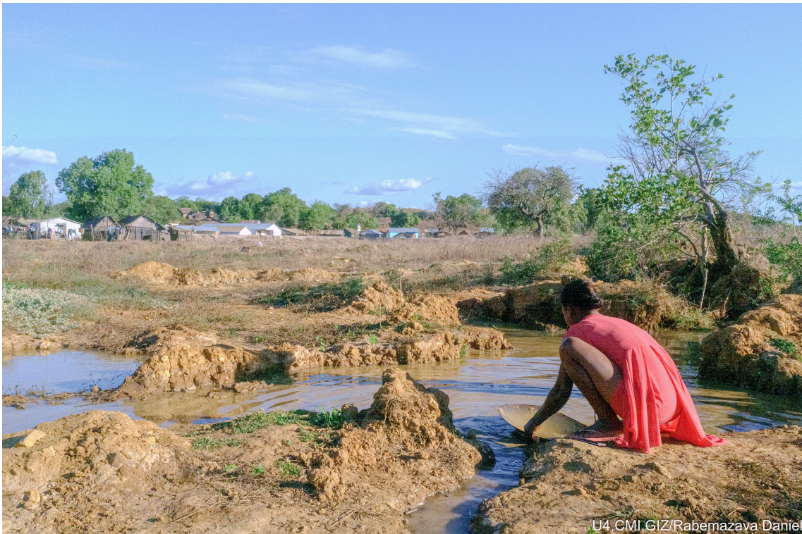
Sieving sand from a pond to find gold (Diana, Betsiaka, Mantelimara sector).
